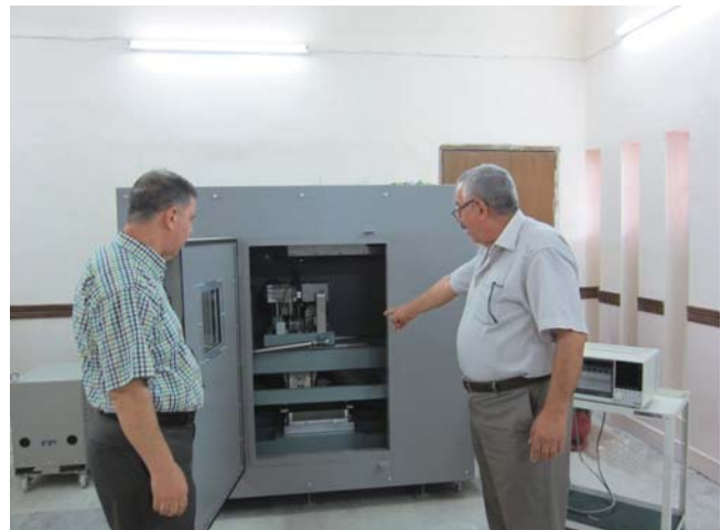
Wheel tracking device that was sent from Japan and installed in PRDC: Mr. Maher B. Antwan, Senior Chief Engineer at PRDC and leader of the project on the Iraqi side (left)
