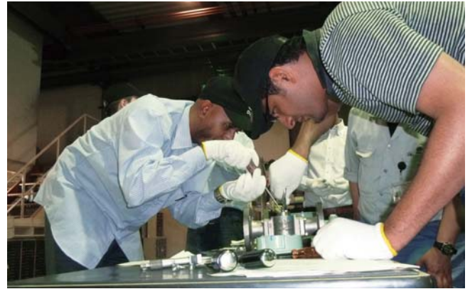
Practical training on the overhaul of a flow meter
