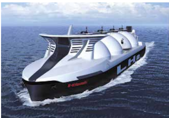
Rendering of a liquefied hydrogen tanker (provided by Kawasaki Heavy Industries, Ltd.)
