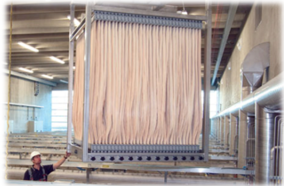
Membrane Bio-Reactor With 80% of wastewater recycling
