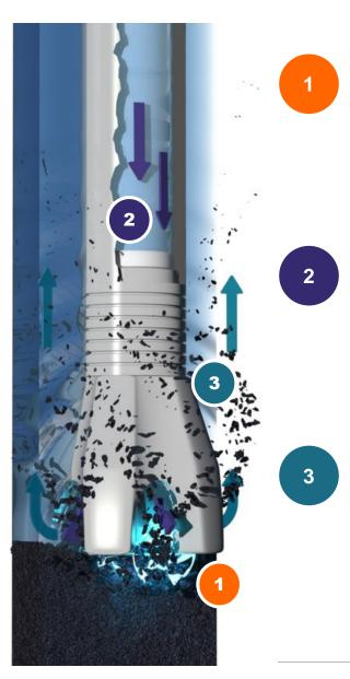
Rock is spalled by repetitive electrical arcs
